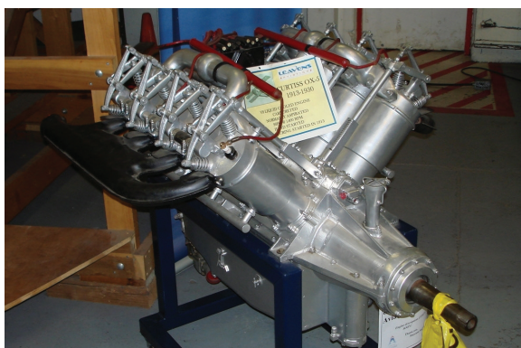
Curtiss OX-5 V-8 Liquid Cooled Engine - Leavens Family Collection Photo - R. Winson
