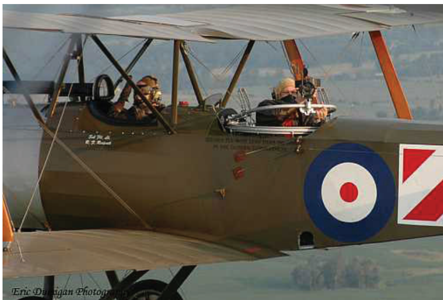
A close-up view showing the Scarff ring-mounted Lewis gun Photo - Eric Dumigan
