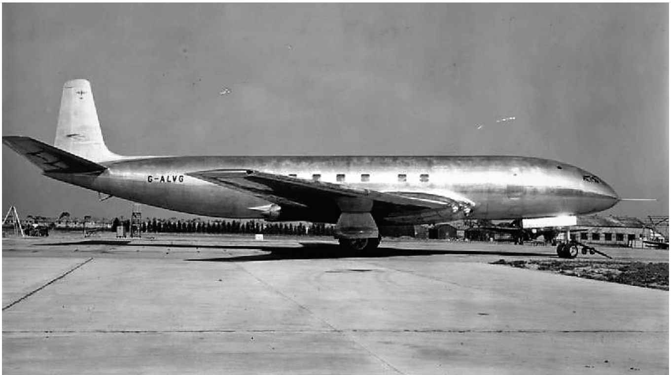
Comet Prototype at Hatfield - Note Square Windows
