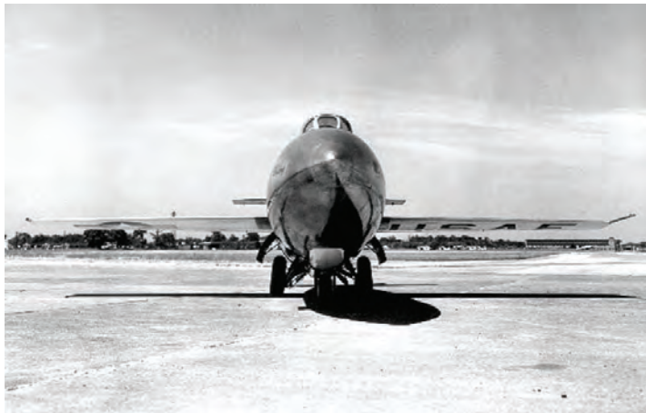
Bell X-1B Front view Showing the duplication of the shape of a 50 cal. bullet Photo Courtesy Bell
