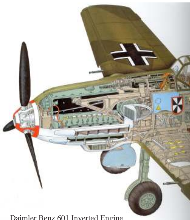
Daimler Benz 601 Inverted Engine Note Supercharger on Left Side Photo - Courtesy Bison Books Ltd.
