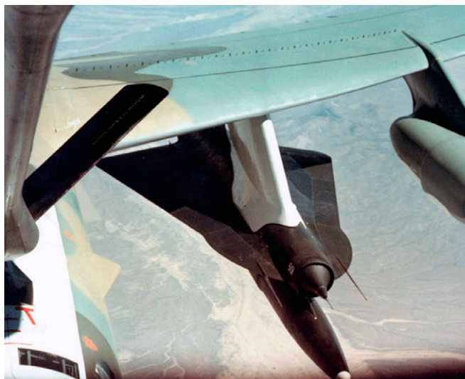
D-21B drone attached to B-52H launch aircraft. Photo National Museum of the USAF.
