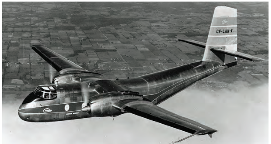
DHC-4 Caribou on test flight - Note wing fences outboard of the port engine. Photo - DHC.
