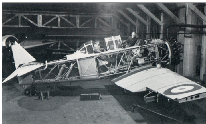
Obsolete tube and fabric construction of a Harvard I is visible during maintenance at Camp Borden c1940.
