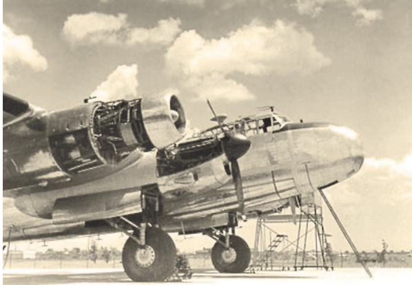
Avro Canada Lancaster 100 FM209 with Outboard Orenda Engines Photo Via Richard Banigan
