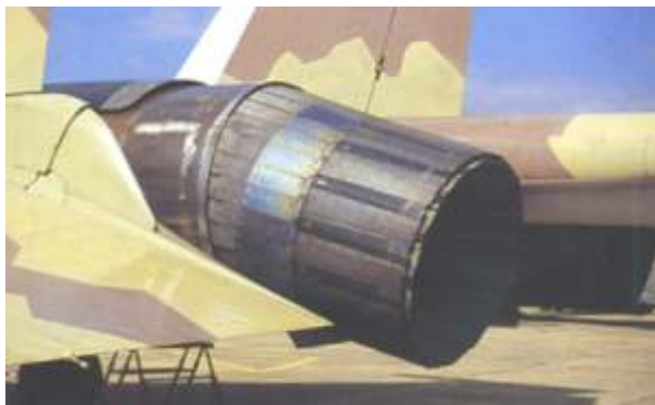
Sukhoi Su-37 Showing two-dimensional thrust vector control engines Photo Credit - www.airforce-technology
