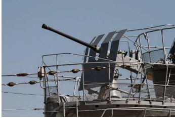
An Anti -Aircraft 3.7 cm 1.5 in. M42 Flak Gun Photo Courtesy - City of Liverpool -Birkenhead - Dario Rich
