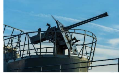
Twin Anti-Aircraft 2 Cm. 0.79 in. C30 Machine Guns Photo Courtesy - City of Liverpool -Birkenhead - Dario Rich
