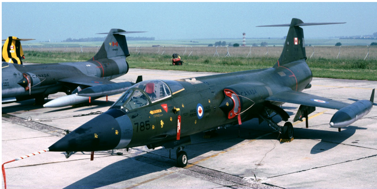
CF-104G Showing Underwing Bomb Racks – Nuclear Weapons were carried on a Centreline Pod • Photo Credit - DND
