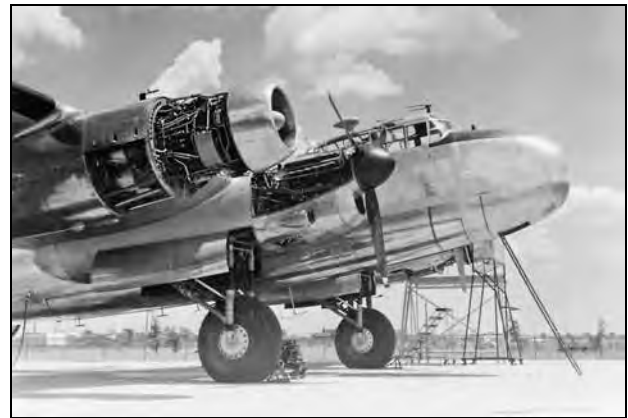
Some of the cowlings around the diverse engines have been removed during a period of ground maintenance on the Lancaster Orenda testbed. (CASM Collection 3601)
