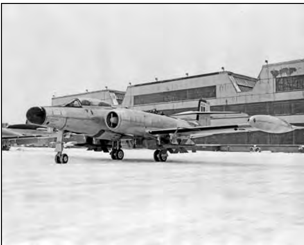
CF-100 Mk 4B serial number 18229 at the Avro Canada facilities is fitted out with four Velvet Glove missiles on their dedicated underwing pylons. In the photo at right, the already cramped cockpit now incorporates additional installations for the Velvet Glove (V.G.). In the right hand corner is the special launcher pylon ("V.G. EXP.-PYLON") umbilical release controls on a bracket. Below and inboard against the windscreen is the "V.G. MISSILE CONTROL/FIRE CONTROL" and the "JETTISON" controls panel.
