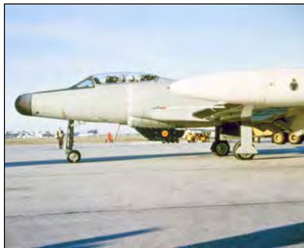
CEPE's CF-100 18434, now in the overall FS 16473 aircraft grey paint scheme due to skin salt corrosion problems, is seen being readied to carry the NASA Nimbus weather satellite's infrared (IR) scanner in February 1964. The black-painted housing for the IR scanner can be seen suspended below the center fuselage in the photo of the aircraft taxiing out from Patrick AFB, Florida for a test run. (George Skinner Collection)
