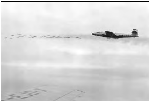
CF-100 Mk 4, 18112 FB-S fires a brace of unguided rockets during flight tests of the ventral pack.
