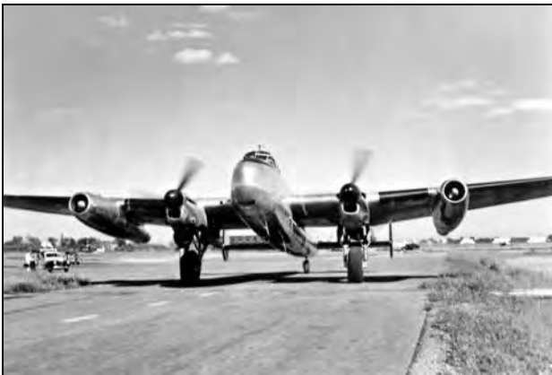
With the Merlin engines running, Avro-built Lancaster Mk X serial FM 209, as the first Orenda engine testbed, taxis out for a test flight. (CASM Collection 3676)
