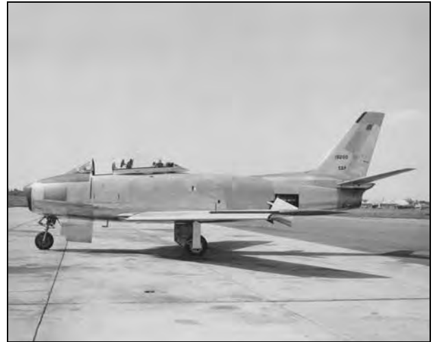
The unpainted Canadair Sabre Mk 3 Experimental Orenda Prototype (E.O.P is seen on the vertical fin) RCAF serial 19200, with an Orenda 3 engine installed, is seen posed on the ramp at Canadair in July 1952. Note the lack of the standard gun blast port panels on the nose. (Canadair via Bill Upton Collection)
