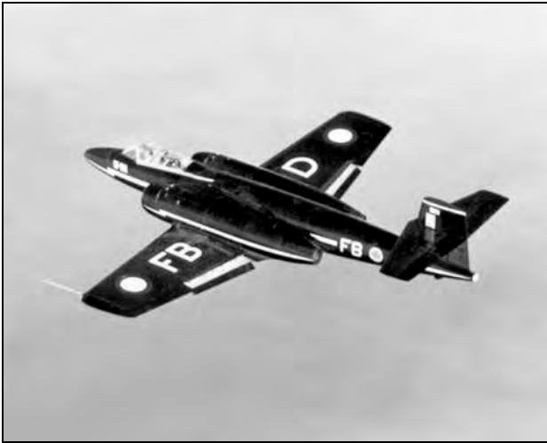
The first prototype CF-100 Mk 1, RCAF serial number 18101 FB-D, during an early test flight in March 1950. Note that the white "CF-100" logo had been applied to each side of the nose once the flight evaluations started.
