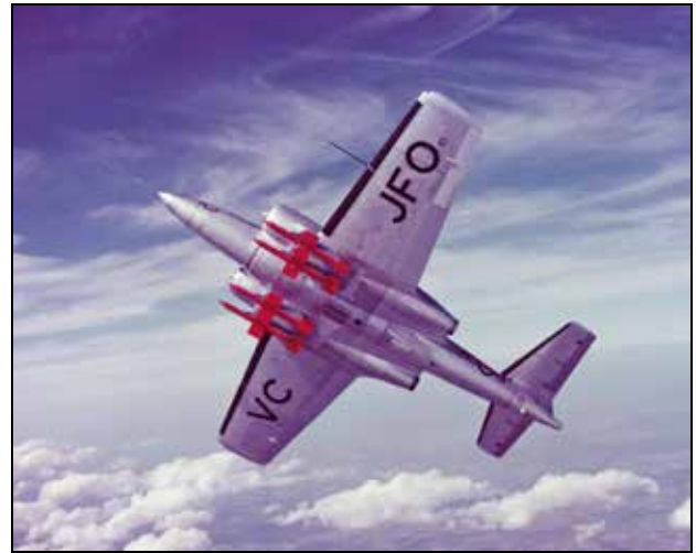
CEPE's CF-100 Mk 3A test aircraft, serial 18117, with four Velvet Glove mockup missiles on under-nacelle pylons in November 1953. The inboard mounted missiles flank the ventral gun pack, the ports of which are visible just forward of the missile's heads. This aircraft evaluated the missile jettison and launch dynamics prior to actual test firings. On 15 October 1954, this aircraft crashed upon takeoff from CEPE Uplands at Ottawa.
