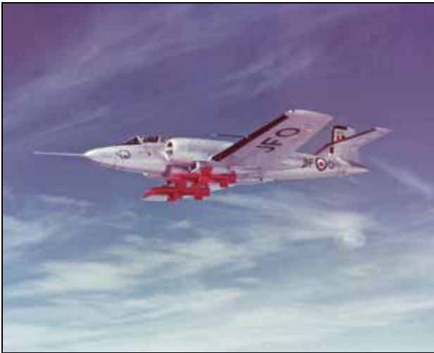
CEPE's CF-100 Mk 3A test aircraft, serial 18117, with four Velvet Glove mockup missiles on under-nacelle pylons in November 1953. The inboard mounted missiles flank the ventral gun pack, the ports of which are visible just forward of the missile's heads. This aircraft evaluated the missile jettison and launch dynamics prior to actual test firings. On 15 October 1954, this aircraft crashed upon takeoff from CEPE Uplands at Ottawa.
