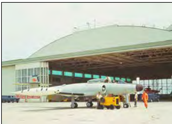
CF-100 18434 of "Operation Lookout" seen with special white wingtip pods carrying sensors and cameras. In the corrosive environment of the coastal areas, oxidization became very apparent on the polished skins of these particular Canadian aircraft. To help remedy this situation and preclude further damage, the local USAF unit graciously repainted the affected Canucks in the USAF's flat grey paint scheme. (George Skinner Photo)
