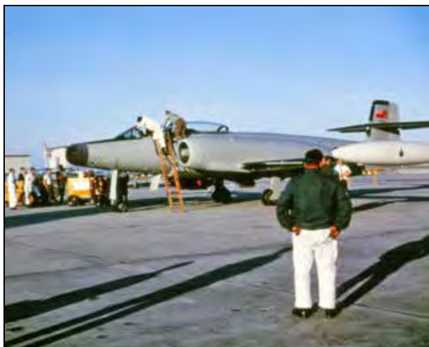
CEPE's CF-100 18434, now in the overall FS 16473 aircraft grey paint scheme due to skin salt corrosion problems, is seen being readied to carry the NASA Nimbus weather satellite's infrared (IR) scanner in February 1964. The black-painted housing for the IR scanner can be seen suspended below the center fuselage in the photo of the aircraft taxiing out from Patrick AFB, Florida for a test run. (George Skinner Collection)
