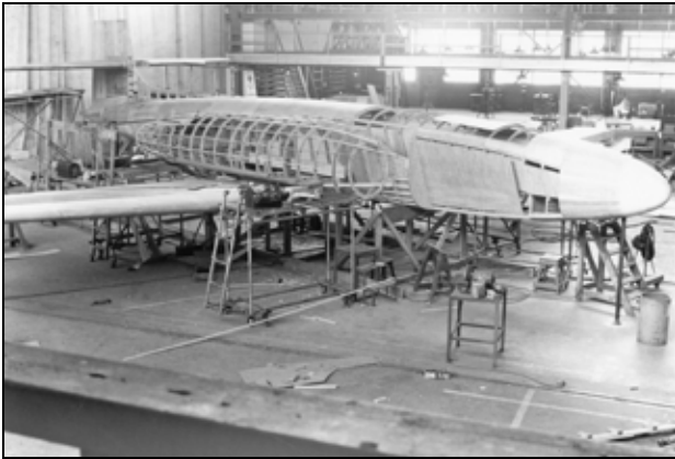
The XC-100 wooden mockup is well advanced in its construction on 3 June 1947. This original design layout of the engine nacelles are slightly higher and positioned further aft above the wings than on subsequent production aircraft. The nacelle repositioning modifications led to later structural problems with the nacelle ring supports. (CASM 28861)
