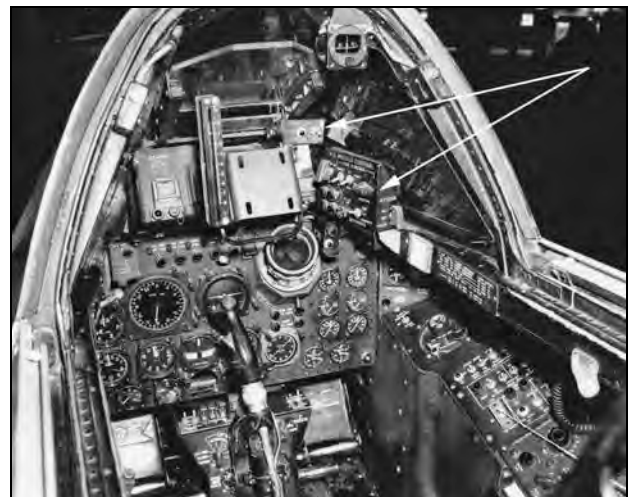
CF-100 Mk 4B serial number 18229 at the Avro Canada facilities is fitted out with four Velvet Glove missiles on their dedicated underwing pylons. In the photo at right, the already cramped cockpit now incorporates additional installations for the Velvet Glove (V.G.). In the right hand corner is the special launcher pylon ("V.G. EXP.-PYLON") umbilical release controls on a bracket. Below and inboard against the windscreen is the "V.G. MISSILE CONTROL/FIRE CONTROL" and the "JETTISON" controls panel.
