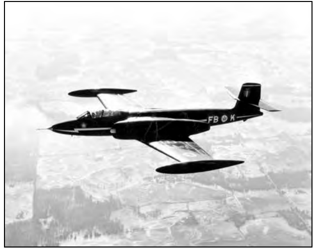
The second CF-100 Mk 1 prototype, RCAF serial 18102 FB-K photographed from the Avro Orenda Lancaster testbed in December 1950, testing the first installation of wingtip fuel tanks. This aircraft had the RCAF heraldic crest on the nose.
